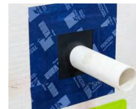
Airtightness grommets need to be used so that service penetrations do not increase air permeability (Source: Pro Clima)
