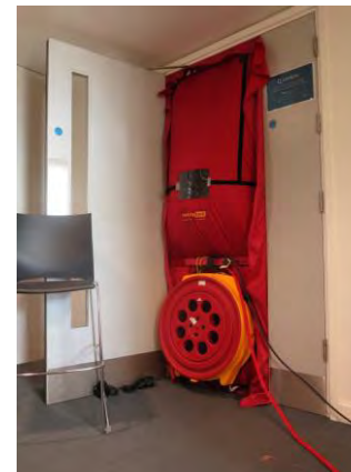
Recommended airtightness process: visual inspection, leak finding and interim air testing are all required before the final air test
